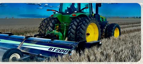
Re-cutter Bar Floating hitch Greasable bearings Cat 3/4 Hitch
